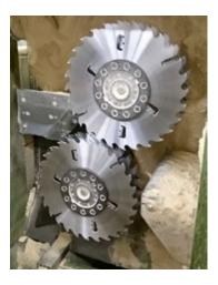
Application at high speed saw mills on double arbor sawing machines such as HewSaw, Linck, AriVislanda, Heinola etc.
